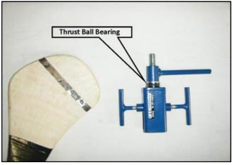
The ideal tool for fitting or re-fitting steel bands on all hurleys.
